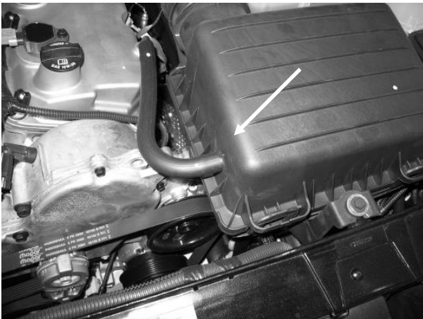
c) Remove the PCV breather tube from the air box.
