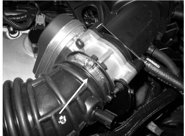
b) Loosen hose clamp at the throttle body.
